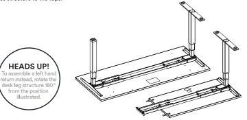
9. Begining at one end, align the bracket holes and leg frame holes with the outermost set of pre-drilled holes on the tops. Install six screws per leg plus two on the G3 leg frame.
