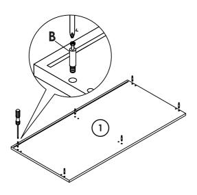
Lower Surface and pins into cam locks Align and tighten cam locks
