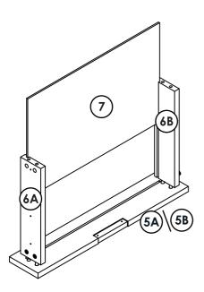
Install, align, and tighten cam locks on to both drawer backs
