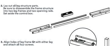
Ensure the proper orientation of leg frame G1
